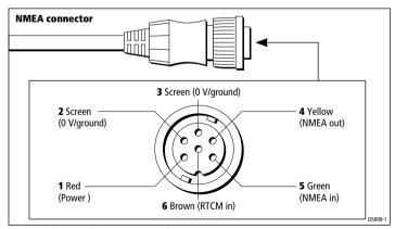
Figure 3-1: NMEA connector pin-outs
