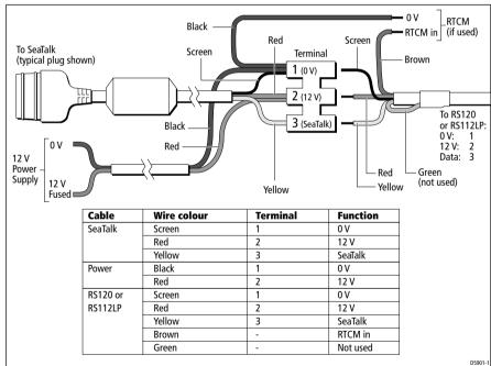
Figure 3-3: NMEA/SeaTalk wiring interconnections
